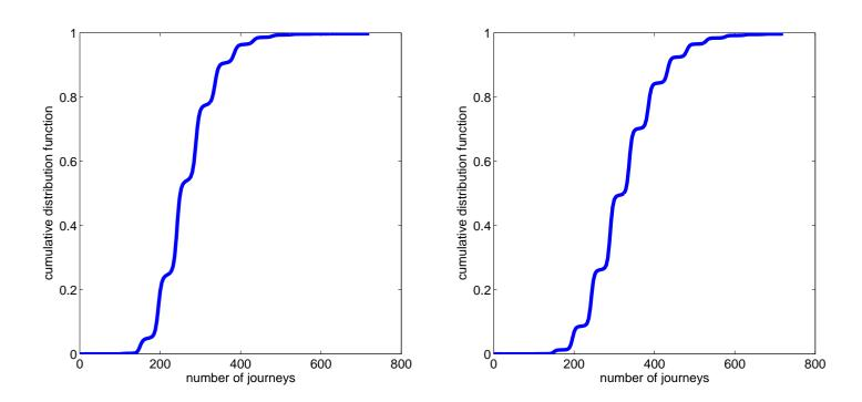
Left: Fatigue life distribution for a vessel with  $\beta = 4$  and  $\log(K) \in N(6.4523 \cdot 10^{-8}, 0.06)$ Right: Fatigue life distribution for a vessel with  $\log(K) \in N(4.5625 \cdot 10^{-7}, 0.06)$
