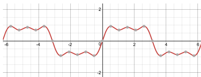
Figur 6.1: Den trigonometriske polynomielle funktion \sin(x) + \frac{1}{3}\sin(3x) + \frac{1}{5}\sin(5x) .
